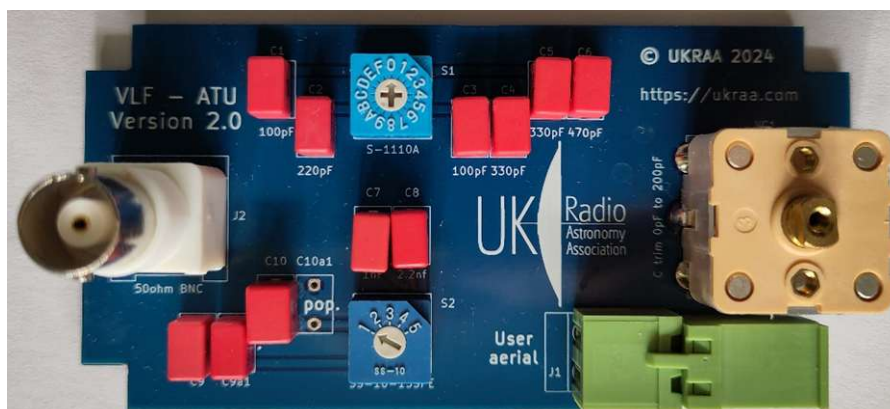
The UKRAA Aerial Tuning Unit Component Layout
