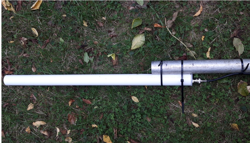
Fig 2 Metal pole mounting, showing overlap of pole and Probe.
