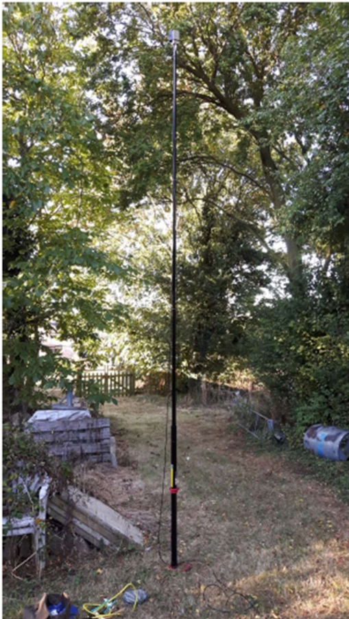
Fig 4 – Probe mounting on temporary fibreglass mast
