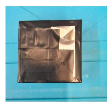
Repeat process; so that there is a **double layer** of PVC tape wrapping the scintillator assembly.
