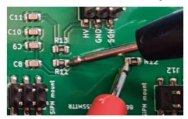
Probe placement on back-side of SiPM PCB.
