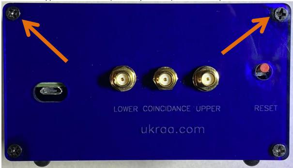
3. Remove the lower x2 case screws (nominally PH2 size) from the front panel.
