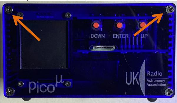
2. Remove the upper x2 case screws (nominally PH2 size) from the rear panel.
