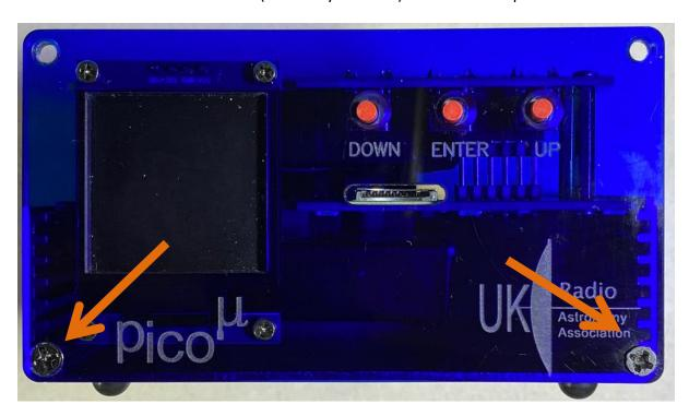
4. The front panel can now be removed from the PicoMuon detector. Pull forward to remove the 1x4 OLED pin header from the 1x4 pin socket located on the upper PCB.
