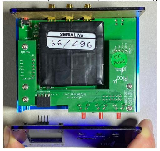
5. Remove the lower x2 case screws (nominally PH2 size) from the rear panel.
