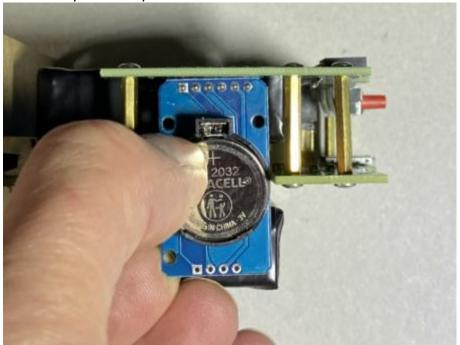
11. Review and ensure that the CR2032 button cell is fully seated into the DS3231 RTC module battery holder.
