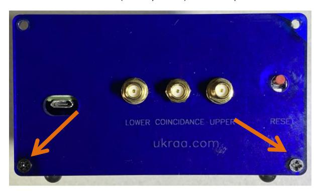
6. Now remove the PCB assemblies from the lower case.
