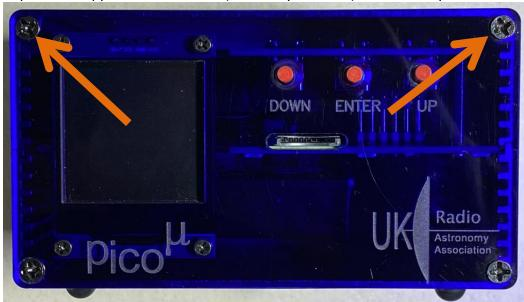
8. Replace the upper x2 case screws (nominally PH2 size) to the rear panel
