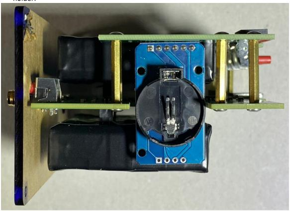
9. Carefully place your CR2032 button cell into the DS3231 RTC button cell holder. Ensure that the + terminal of the button cell is facing out – towards you.
