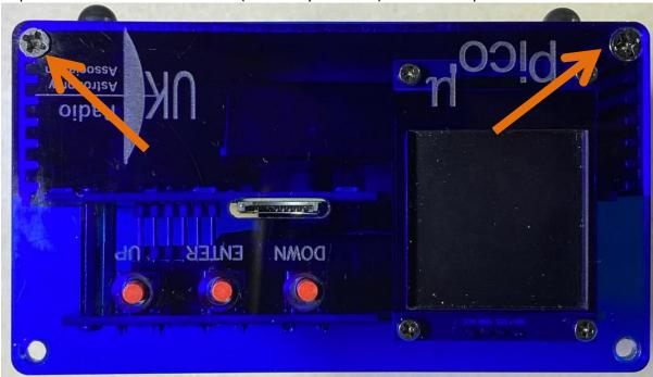
3. Replace the lower x2 case screws (nominally PH2 size) to the rear panel.
