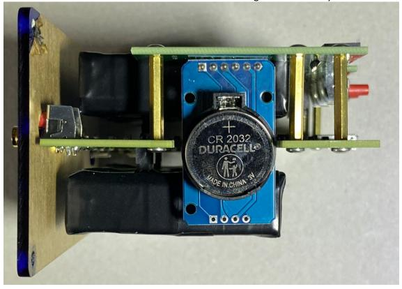
10. Apply pressure to the top of the CR2032 button cell, while supporting the bottom of the DS3231 RTC module, until the CR2032 button cell is fully seated in the DS3231 RTC battery holder – you will hear a click.
