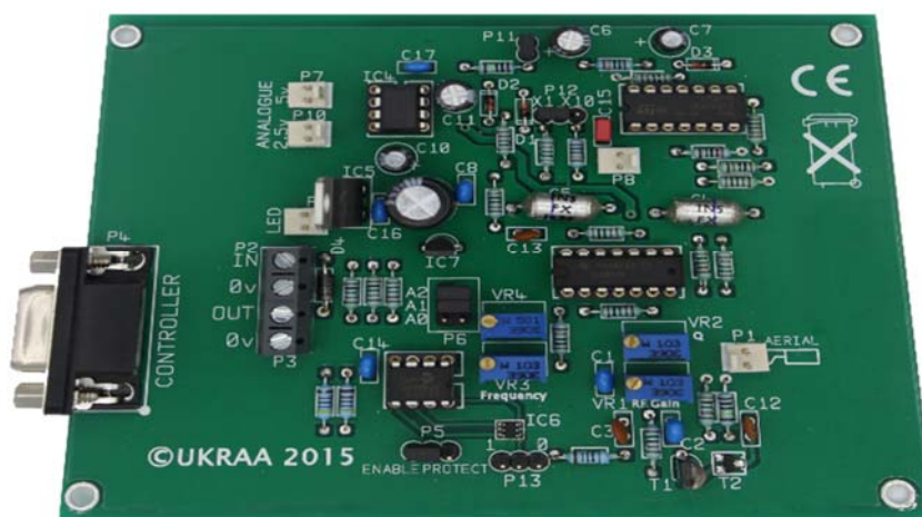
The UKRAA VLF Receiver Circuit Board
