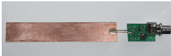
PCB plate attached to antenna
