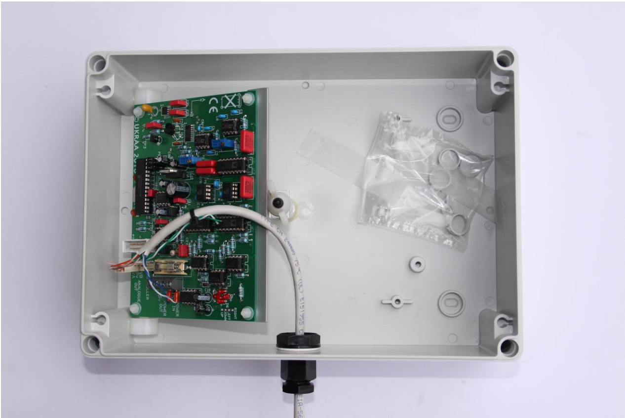
Figure 2 UKRAA Magnetometer in custom enclosure
