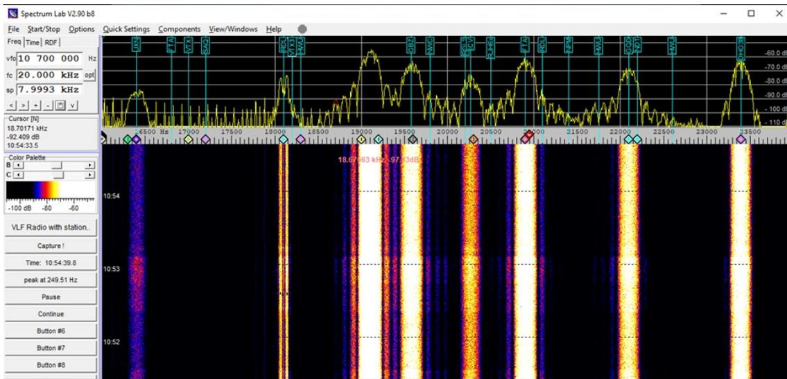
EFP Antenna Signals                      19.1kHz    19.6kHz    20.9kHz    22.1kHz    23.4kHz
