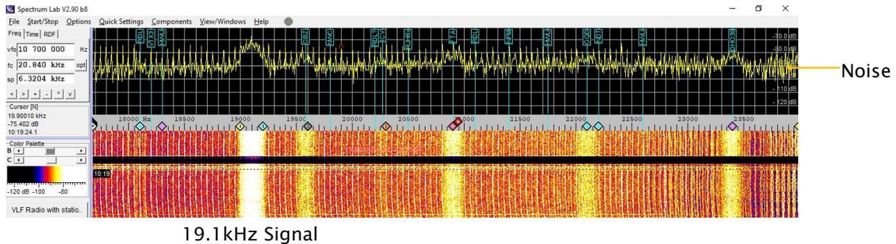
Spectrum Lab trace showing signals barely detectable above the noise.
