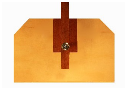
Clamp side plate with frame guide strip
