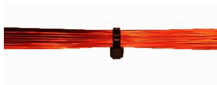
Cable tie applied to windings
